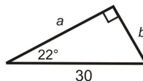
We are given the hypotenuse. Use sine ( $\frac{\text{opposite}}{\text{hypotenuse}}$ ) to find  $b$  and cosine ( $\frac{\text{adjacent}}{\text{hypotenuse}}$ ) to find  $a$ . Use your calculator to evaluate the sine and cosine of the angles.
