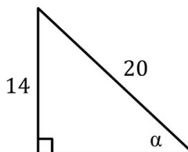
$$\begin{aligned}\sin \alpha &= \frac{14}{20} \\ &= 0.7 \\ \alpha &= \sin^{-1} 0.7 = 44.4^\circ\end{aligned}$$
