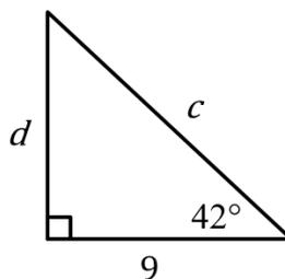
We are given the adjacent length to the angle of  $42^\circ$ . Use cosine ( $\frac{\text{adjacent}}{\text{hypotenuse}}$ ) to find  $c$  and tangent ( $\frac{\text{opposite}}{\text{adjacent}}$ ) to find  $d$ .
