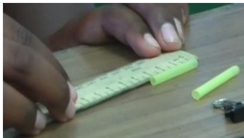
A student correctly aligning the zero on a ruler to measure length
