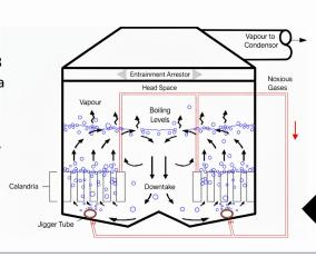
The jigger system design enhances vacuum pan performance by utilising waste heat in a precision injection system to improve circulation and heat transfer.
