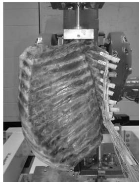
Right: Six degree of freedom spine testing robot used to test calf spine & ribcage with an Optotrak Certus motion tracking system.
