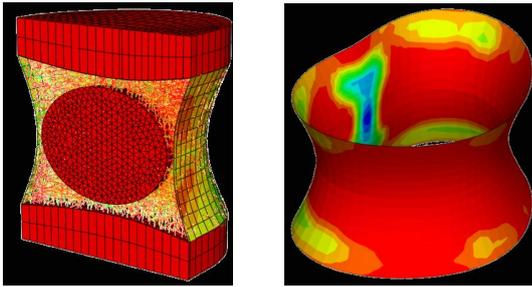
(Left) Computer model of an osteoporotic vertebra augmented with bone cement and (Right) Computer model predicting bone strains in the outer shell of an osteoporotic vertebra under body weight loading.
